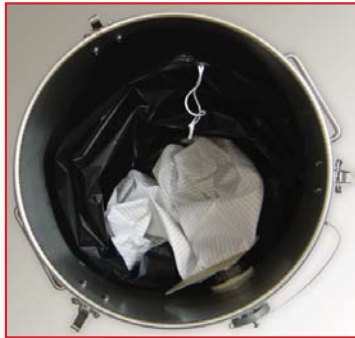
Potent compounds and powders are recovered into a static dissipating disposable cloth filter bag placed within a conductive polyliner
