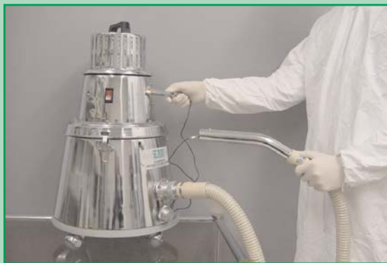
Fig. 1 Ground tester to verify continuity
